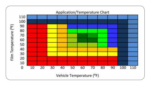
Install Not Recommended at temp. Cool down car or film by spraying cold water on vehicle surface.
