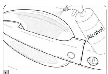
Prep surface for film placement. Alcohol entire area and place film into door cup.
