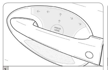
Using your thumb press down in center of the door cup, move upwards and out, fastening the sides of the film down.
