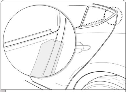
Door edges will be installed dry, **(NO ALCOHOL)** match the "V" cut in film to the edge of the door as shown in picture. It should be somewhere in the middle, enough to wrap around the door. Once aligned apply pressure to film.
