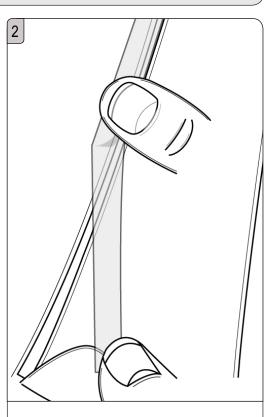
With door closed use the inside edge of film with the other door's edge to help align and place the strip onto the outside of the door edge.
