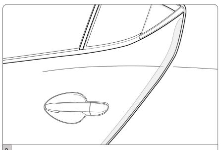
Once film is aligned to door edge surface open door and half of the film strip should hang over. Using your finger gently stroke hanging film inward, slowly and cautiously until entire edge is positioned in place.
